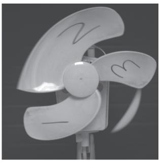
Figure 2. Example of the distortion produced by a rolling shutter when the reading speed is on the order of the speed of the photographed object. Left: Global shutter. Right: Rolling shutter. Image credit: Andor and Oxford Instruments Company.
