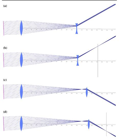
**Fig. 4** Refracting telescopes in direct view and projection mode. **a** Galilean telescope when looking through it, **b** Galilean telescope when projecting the image, **c** Keplerian telescope when looking through it, and **d** Keplerian telescope when projecting the image. Images based on the ray-tracing by https://ricktu288.github.io/ray-optics/
