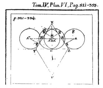
Fig. 18 Rhomb-shaped cross-hairs for measuring positions in the eyepiece as described by Flaugergues (1813)
